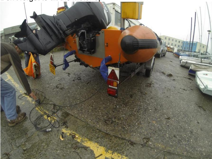
2/. Ensure the painter is secured to the end to the post that holds the winch (make sure the winch handle is available). Remove electrics
