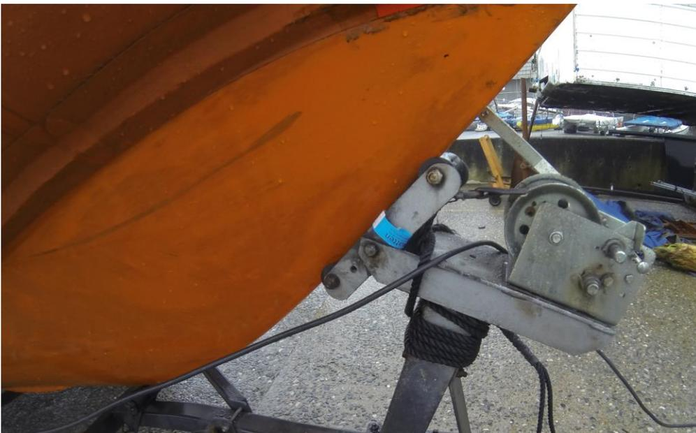
4. Carefully uncoil the painter and remove from the post – maintain tension!
