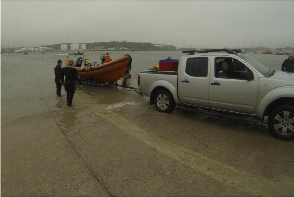
3. Detach the winch line from the bow attachment point
