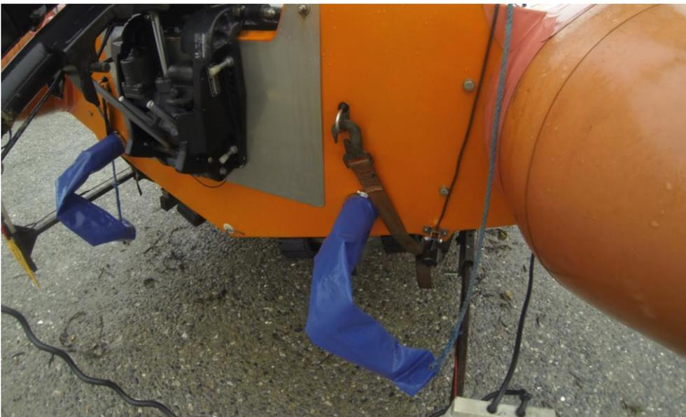
6. Tow the trailer off the slip and re- attach the retaining straps and lighting boards
